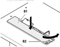
11. Turn the countersunk screw (82) counter-clockwise against the stop.
